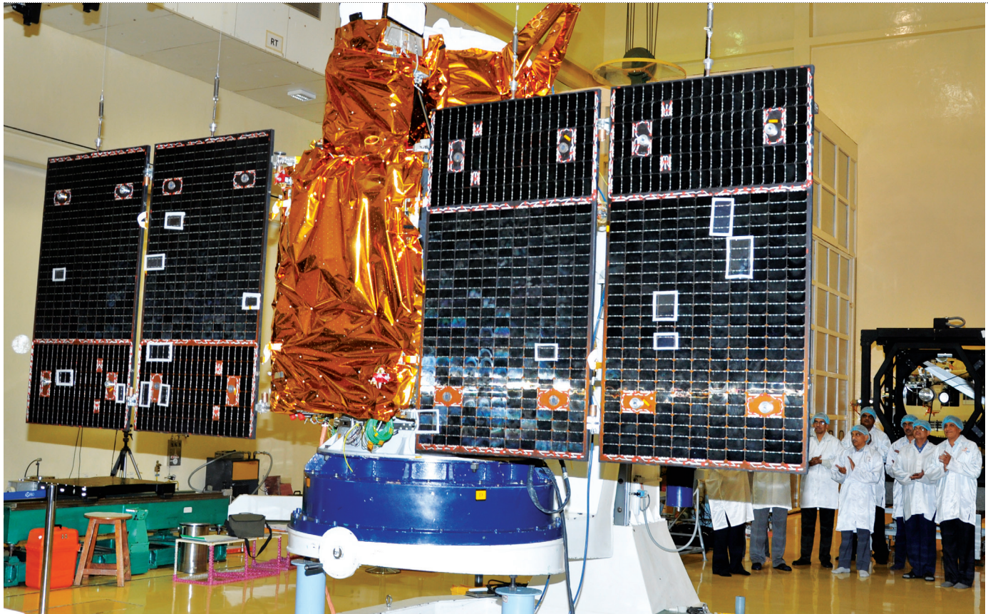
Two solar panel deployment test at Bengaluru
